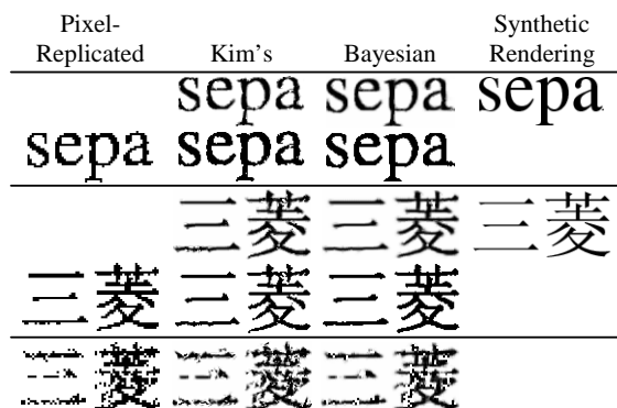
Fig. 4. Selected Results: These are small clippings from three tests. We used Kim's method and our Bayesian method for super-resolution, with 5 \times 5 low-res patches and non-overlapping 2 \times 2 high-res patches. The input to the first two rows is from an English document, using 12pt. Times New Roman, scanned in at 200dpi. The next two rows are from a Japanese (Kanji) document, using 12pt. SimSun, also scanned at 200dpi. The final row is the same as the previous pair, except the data were generated by rendering the image with synthetic noise and the Bitstream Cyberbit typeface was used. The bilevel images (2 nd and 4 th rows) were created by manually selecting a threshold on the corresponding grayscale images.
