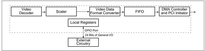
Figure 29. GPIO Normal Mode
