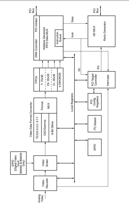
Figure 1. Bt848/848A/849A Detailed Block Diagram
