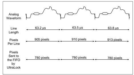
Figure 4. UltraLock Behavior for NTSC Square Pixel Output
