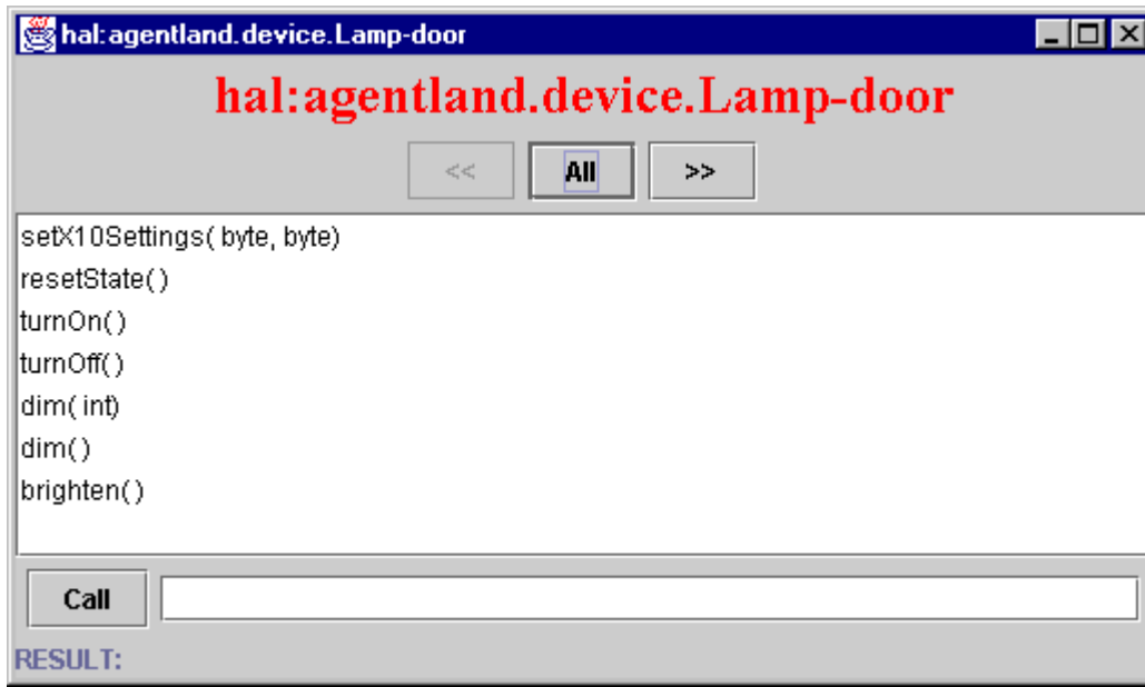
Figure 3.4 – The Agent Tester agent allows for any Metaglu agent to be launched and any method called. Above, a window for controlling the lamp by the door pops up per request.
