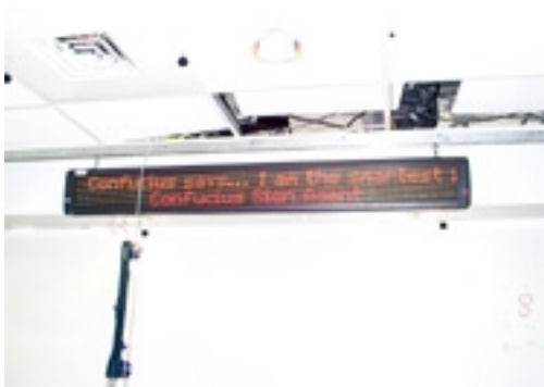
2.1.e – Alpha LED display, which displays textual data.
