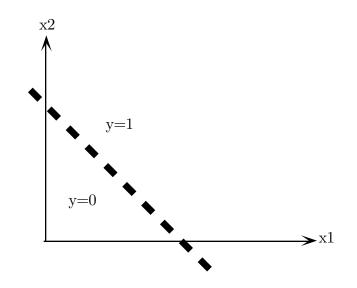
where  $x_i$  are the input variables and  $w_i$  are the weights. Alternatively, as a matrix equation, we have that the dot product of  $[x_1s_2]$  and  $[w_1w_2]$  is equal to the constant 0. This is true of the points on the line perpendicular to the vector  $[w_1w_2]$ . If we let w be the length of the vector  $[w_1w_2]$ , i.e.,  $\sqrt{w_1^2 + w_2^2}$ , then we can write this as:
