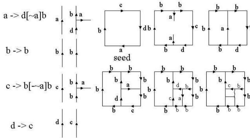
**Fig. 3.** An example of a Map L-System from [8]. The rewrite rules are shown to the left in symbolic and graphical form. Next, the seed (a square) is shown and the rewrite rules are subsequently applied to it.
