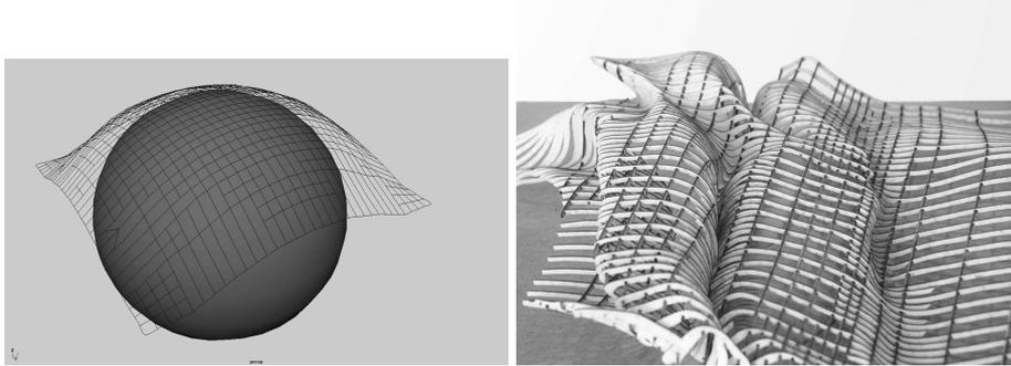
**Fig. 1.** Left hand side, a Genr8 surface grown in an environment where it has been pulled down by gravity on top of a spherical boundary. Right, a physical model made by Jordi Truco at the Architectural Association in London. The design process started with Genr8 and the evolved digital surface was subsequently exported so that a physical model could be manufactured.
