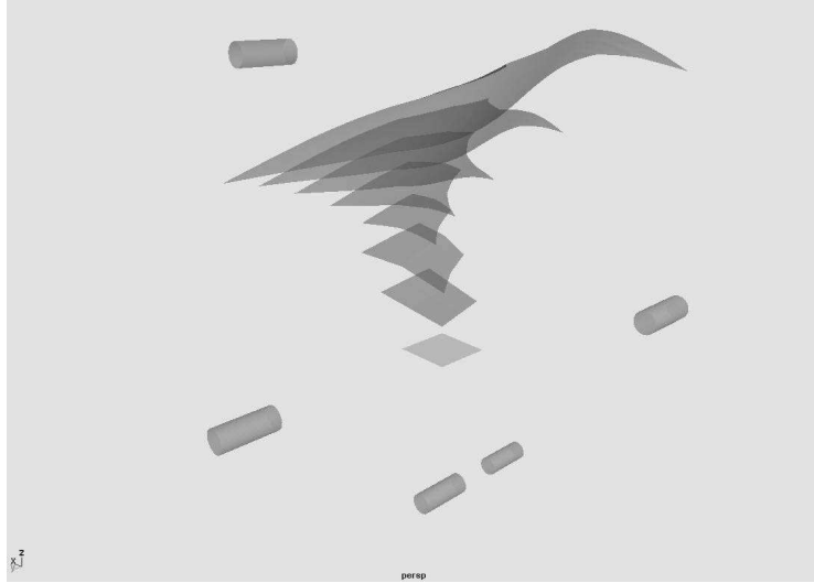
Fig. 4. A time series capturing 7 growth steps of a HEMLS surface in an environment with five repellers (here drawn as cylinders). The smallest surface is the axiom. The largest surface is the final growth step.
