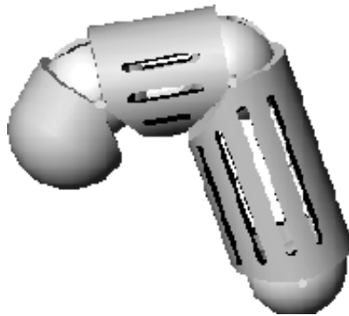
Figure 1: SolidWorks assembly of robot finger. Actuators and sensors not included.
