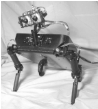
Figure 1: Coco a 15 dof ape-like robot.
