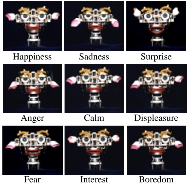
Figure 2: Kismet, a robot capable of conveying intentionality through facial expressions and behavior.
