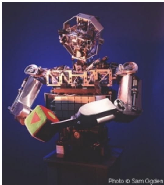
Fig. 3. Cog, an upper-torso humanoid robot with twenty-one degrees of freedom and sensory systems that include visual, auditory, tactile, vestibular, and kinesthetic systems.
