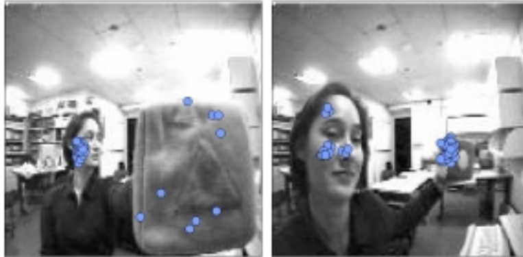
Fig. 9. Effect of gain adjustment on looking preference. Circles correspond to fixation points, sampled at one second intervals. On the left, the gain of the skin tone filter is higher. The robot spends more time looking at the face in the scene (86% face, 14% block). This bias occurs despite the fact that the face is dwarfed by the block in the visual scene. On the right, the gain of the color saliency filter is higher. The robot now spends more time looking at the brightly colored block (28% face, 72% block).
