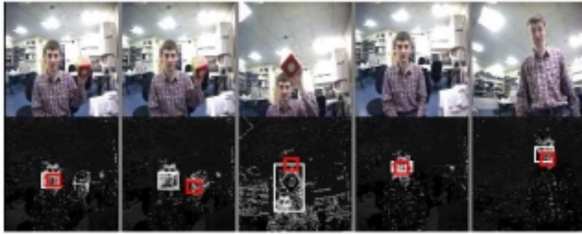
Fig. 8. Manipulating the robot’s attention. Images on the top row are from Kismet’s upper wide camera. Images on the bottom summarize the contemporaneous state of the robot’s attention system. Brightness in the lower image corresponds to saliency; rectangles correspond to regions of interest. The thickest rectangles correspond to the robot’s locus of attention. The robot’s motivation here is such that stimuli associated with faces and stimuli associated with toys are equally weighted. In the first pair of images, the robot is attending to a face and engaging in mutual regard. By shaking the colored block, its saliency increases enough to cause a switch in the robot’s attention. The third pair shows that the head tracks the toy as it moves, giving feedback to the human as to the robot’s locus of attention. The eyes are also continually tracking the target more tightly than the neck does. In the fourth pair, the robot’s attention switches back to the human’s face, which is tracked as it moves.
