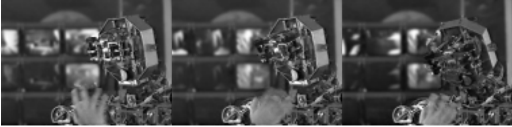
Fig. 5. Orientation to a salient stimulus. Once a salient stimulus (a moving hand) has been detected, the robot first saccades to that target and then orients the head and neck to that target.
