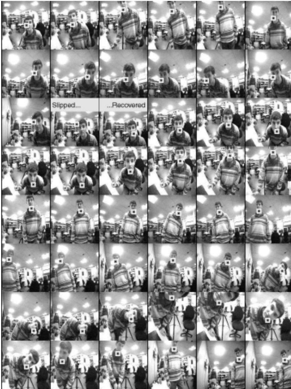
Fig. 11. Behavior of the tracker. Frames are taken at one second intervals. The white squares indicates the position of the target. The target is not centered in the images since they were taken from a camera fixed with respect to the head. On the third row, the face slips away from the tracker, but it is immediately reacquired through the attention system. The images are taken from a three minute session during which the tracker slipped five times. This is typical performance for faces, which tend not to move too rapidly.
