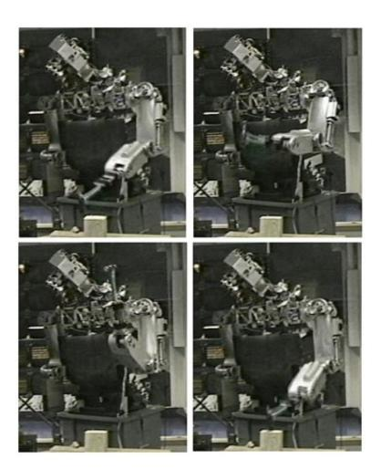
Figure 7-19: **REAL** Four stills from a video of the robot hammering a nail. The sequence goes from left to right and top to bottom. The elbow and shoulder joints drive up and down to give a powerful hit with the hammer. The motion causes the hammer to be swung fairly high, and extend the wrist joint (lower left picture). This stored energy is then released into the nail (lower right).
