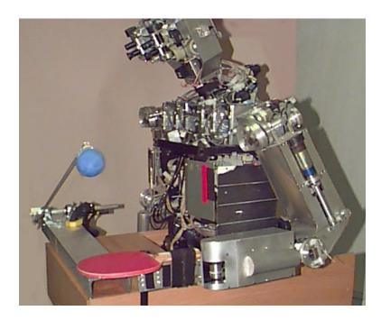
Figure 3-20: Picture of robot in juggling task. The paddle is a table tennis bat attached to the robot's arm. The ball is restrained to travel in one dimension by being mounted on a rotating boom. The angle of the boom is measured using a potentiometer at the pivot point, and this feedback signal is used by the oscillator to coordinate the arm motion with the ball motion.
