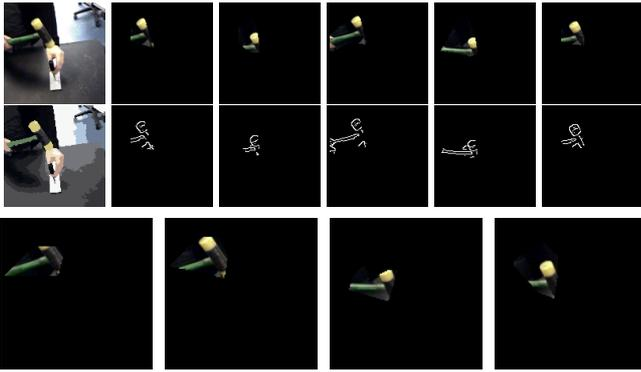
Figure 12: Results for the segmentation of an hammer. Each sequence of images of size  $n$  originate  $n$  templates for an object. The top row shows 5 templates for five frames along the trajectory. The middle row shows the edge images using a Canny edge detector. The bottom row shows four hammer templates obtained from four different image sequences.
