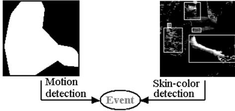
Figure 4: An event detection is triggered by a minimum number of moving points and a minimum number of actuator points in the image at a given time instant.
