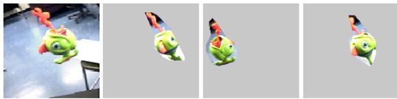
Figure 9: The left image shows a pendular object immediately after being poked by the robot. The other images show object segmentations for three different runs.
