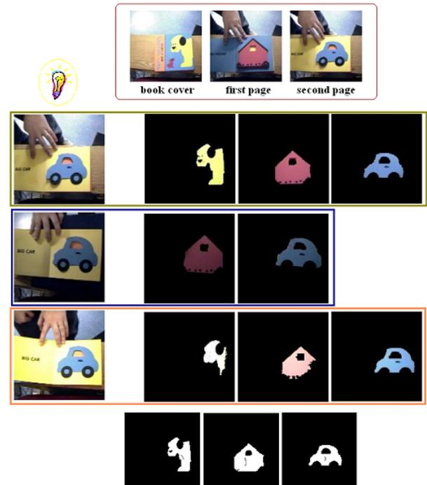
Figure 13: The top images show three different pages of a book. The bottom images show the masks obtained with the actuator trajectory on it. The other rows of images show segmentations for different luminosity conditions.
