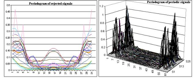
Figure 5: The left graph shows the WFFTs of discarded points, while the right image displays the WFFTs for a set of points contained on an object moving periodically.
