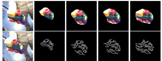
Figure 8: Top row: A image of the scene is shown on the left image, while object templates for the 1<sup>st</sup> image of the images sequence are shown in the right. Bottom row: Color segmentation of scene on the left, and edge masks of templates obtained by a Canny edge detector.
