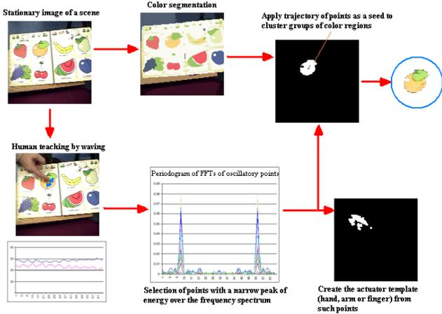
Figure 6: The algorithm works as follows: a human teacher waves on top of the object to be segmented. The motion of the actuator is tracked and the energy per frequency content is determined. A template of the actuator is built from the set of periodic moving points, while the trajectory is used to segment the object from the color segmentation image.
