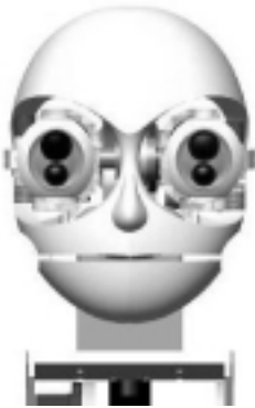
Figure 4: The first prototype of Cog's face as implemented via solid modeling. This is a SolidWorks image.
