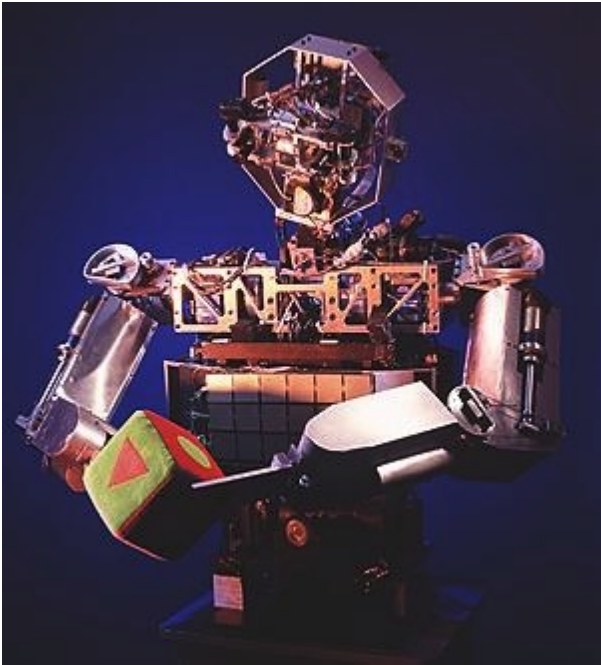
Figure 1: Our upper-torso development platform, Cog, has twenty-two degrees of freedom that are specifically designed to emulate human movement as closely as possible.
