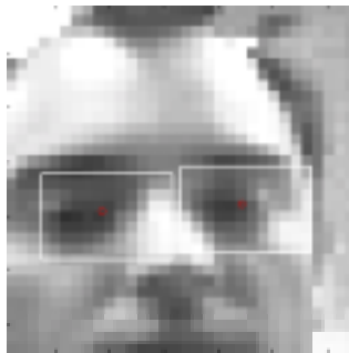
Figure 6: Eyes are searched for within a restricted part of the robot's field of view.
