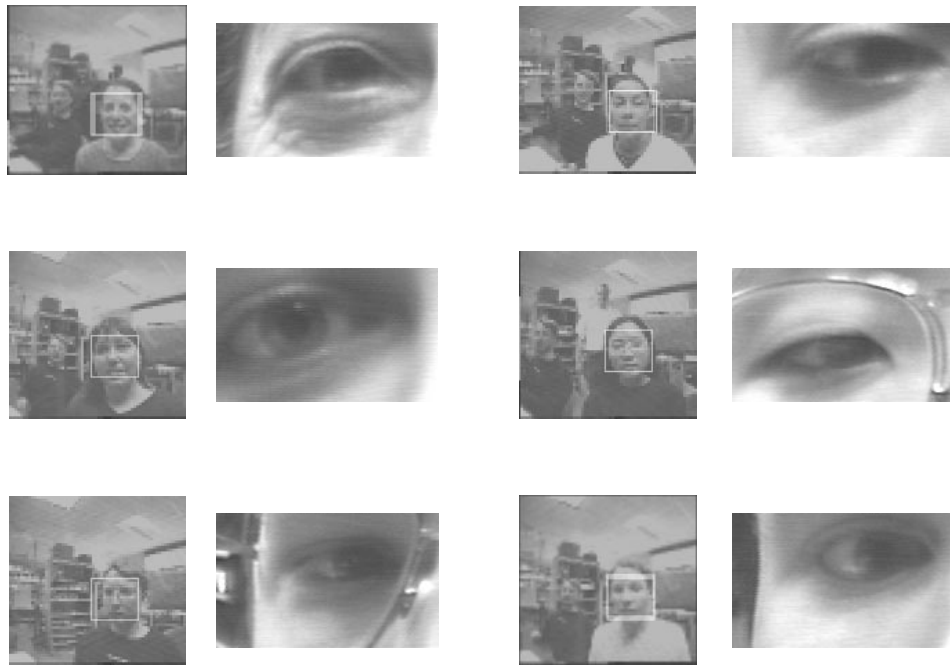
Figure 7: Additional examples of successful face and eye detections. The system locates faces in the peripheral camera, saccades to that position, and then extracts the eye image from the foveal camera. The position of the eye is inexact, in part because the human subjects are not motionless.
