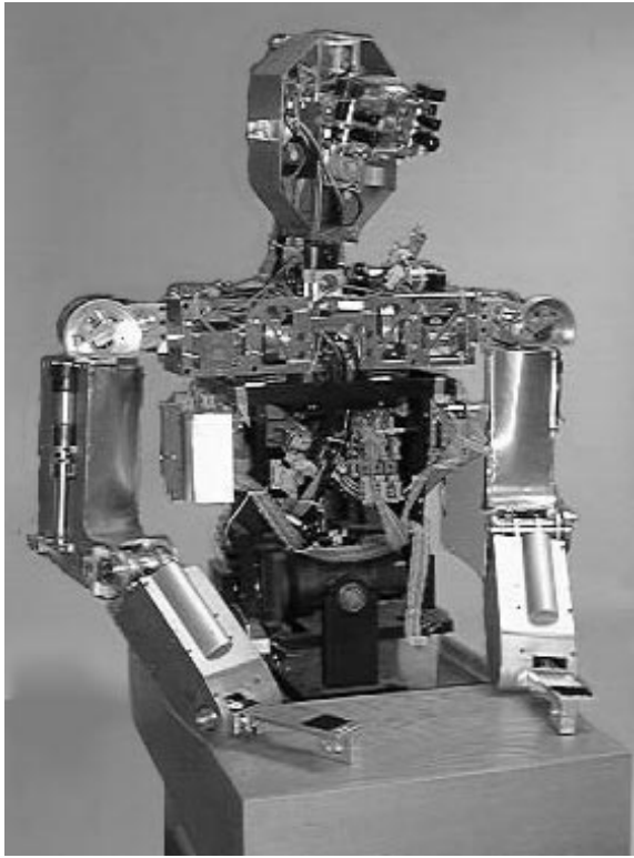
Figure 3: Cog, an upper-torso humanoid robot with twenty-one degrees of freedom and a variety of sensory systems including visual, auditory, tactile, kinesthetic, and vestibular systems.
