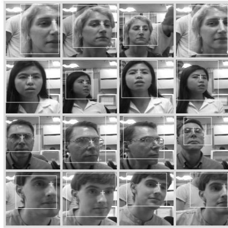
Fig. 12. Eyes are searched for within a restricted part of the robot’s field of view. The eye detector actually looks for the region between the eyes. It has adequate performance over a limited range of distances and face orientations.
