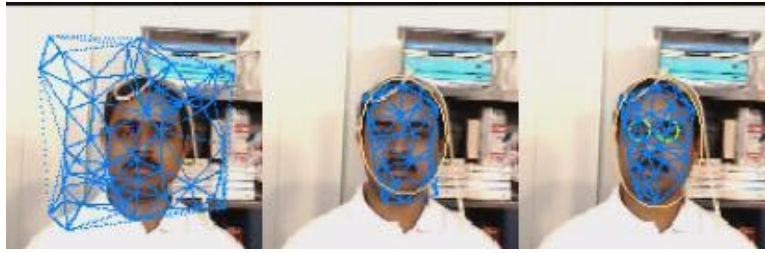
Fig. 8. Mesh initialization (apologies if you are viewing this in grey-scale). The mesh is initially distributed arbitrarily. It is pruned by the head outline when it is detected, and by heuristics based on the relative motion of different parts of the mesh. When frontal pose is detected, surface coordinates of the mesh can be initialized within the parallel region (that part of the face that is parallel to the image plane).
