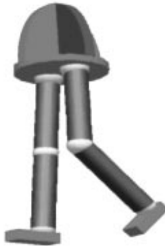
Figure 4: Three Dimensional bipedal walking simulation. The robot has twelve degrees of freedom: three in each hip, one in each knee, and two in each ankle.
