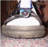
Figure 1. The system. A camera and inertial sensor are mounted on a sandal.
