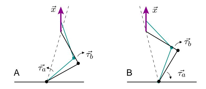
(B) Joint a applies torque  $\vec{\tau}_a$  in opposition to its displacement.
