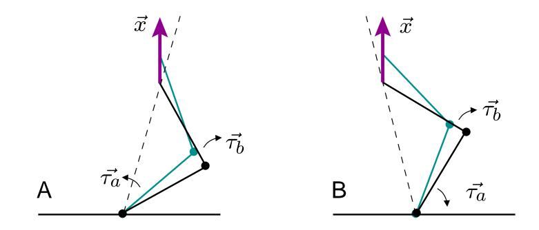
To do work along  $\vec{x}$  — that is, to apply a force along that vector — the arm must move into the blue configuration.
