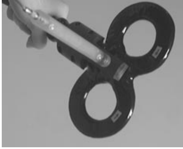
Figure 17: Stimulation coil used for TMS mapping. Note the rod mounted orthogonal to the plane of the coil—two LEDs are fixed on the rod for tracking the position and orientation of the coil.
