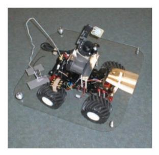
Radio-controlled vehicle. This is a small (50 x 50 x 50 cm) wheeled platform with electric motor, spring-based suspension system, and radio-controlled steering and throttle.
