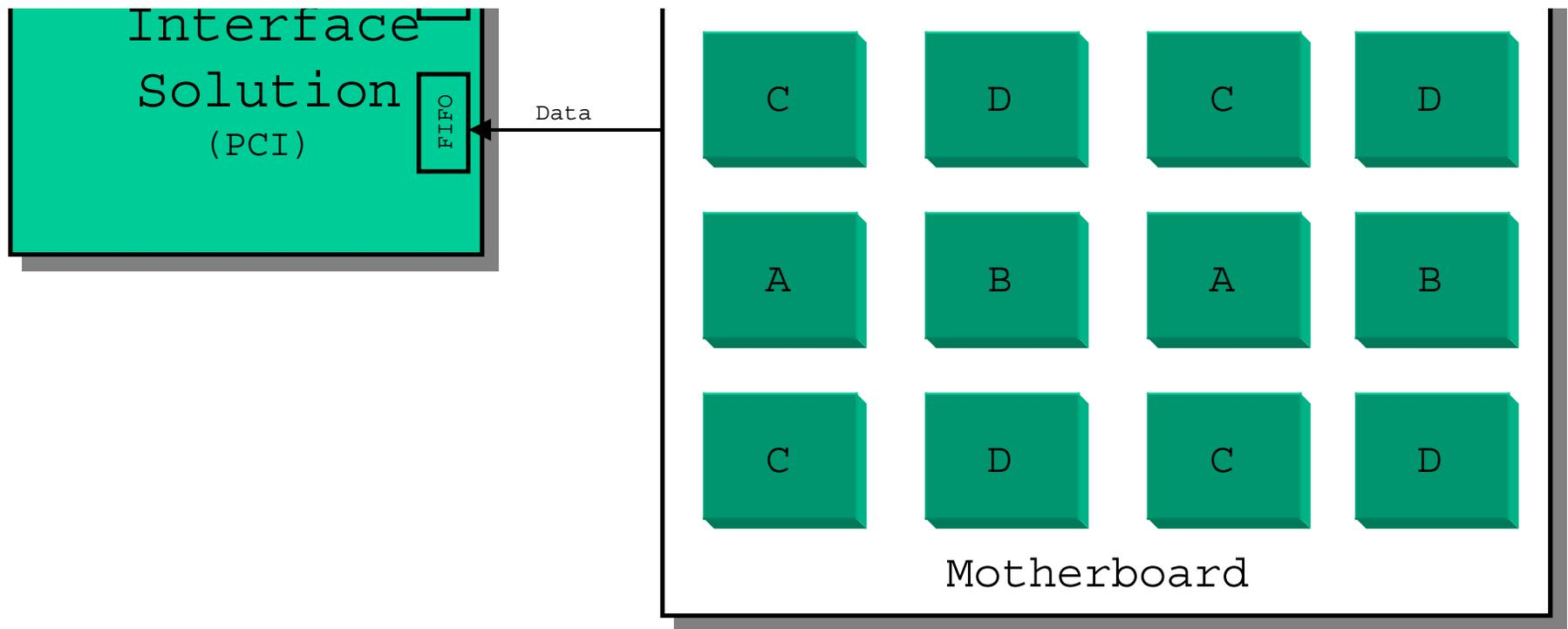
A high-level block diagram of our proposed system is shown above. The camera's most interface will be an industry standard personal computer bus. The camera will be constructed from modular sensor units mounted on a common mother
