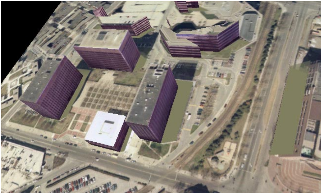
Figure 6. Result of reconstruction: a textured geometric model representing the office park.
