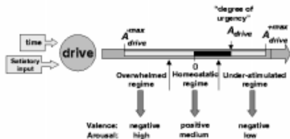
Figure 4: Kismet’s affective state can be influenced by the drives. The overwhelmed regime has an agitating effect, the homeostatic regime has a calming effect, and the under-stimulated regime has a depressing effect.
