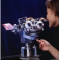
Figure 3: Appearance-wise, Kismet has been designed to have an infant appearance according to the ‘baby-scheme’ of Eibl-Eibesfeld (address design Issue I). Specifically, Kismet has large eyes, a demure chin, lips suggest the ability to suck, and the suggestion of a high forehead.
