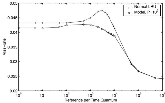
**Fig. 11.** The results of the model-based cache partitioning for a set-associative cache when eight processes (*bzip2*, *gcc*, *swim*, *mesa*, *vortex*, *vpr*, *twolf*, *iu*) are sharing the cache (32 KB, 8-way associative).
