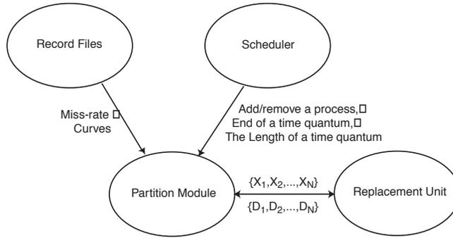
**Fig. 8.** The implementation of on-line cache partitioning.
