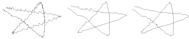
Fig. 1. A very noisy stroke along with the fits generated using curvature and speed data with average based filtering. Both fits have picked many false positives due to noise.
