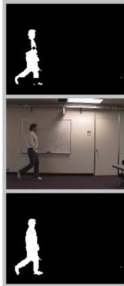
Figure 1: Top: The result of segmenting the human body from the stationary background is not perfect, as this example illustrates. Middle: This is the frame to which the body tracking system will fit the body model. Bottom: This is an example of a projection of the human model fitted to a frame.
