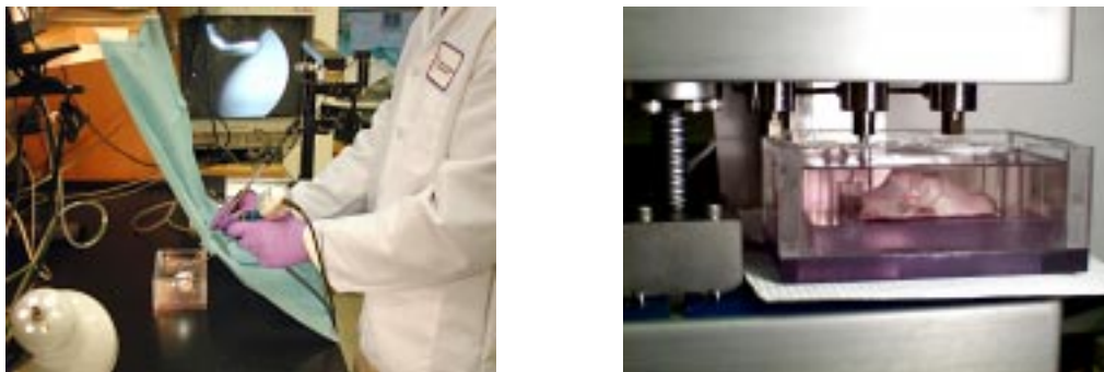
Figure 1: left Surgical probe (seen held in right hand) instrumented with strain gages and 6 DOF position tracking is used to examine the cartilage surface of a tibial plateau. The arthroscope (held in left hand) view is shown on the monitor in the background—the probe tip is visible as it touches the cartilage surface. right The sample is immersed in saline solution and placed on the stationary platform of the compression apparatus. A rigid indenter, affixed beneath a load cell, can be seen just touching the cartilage surface as computer-controlled displacements are applied and the resulting load signal is recorded.
