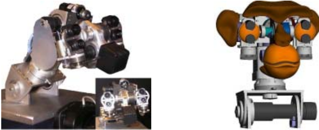
Figure 1: Macaco: the dog-like (left) and primate-like (right) robotic heads. The mechanical design was carried on CAD tools, and the primate-like face was built through a Dura-forming process.
