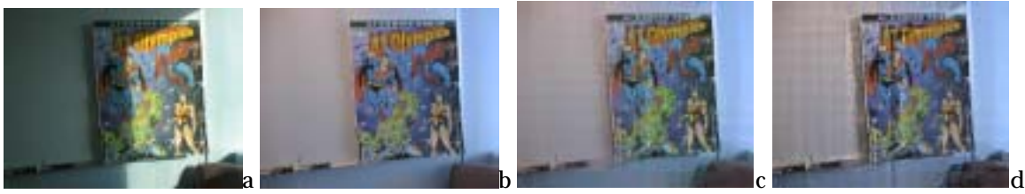
Figure 2: a. Image with strong shadow. b. The same image under more uniform lighting conditions. c. Flow from a to b using piecewise color flows. d. Flow from a to b using another common algorithm in a piecewise fashion.
