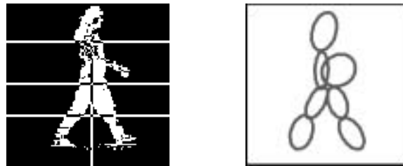
Figure 3: The silhouette of a foreground walking person is divided into 7 regions, and ellipses are fitted to each region.
