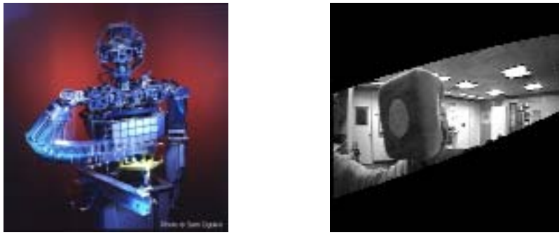
Figure 1: Humanoid robot Cog executing a task - turning a crank (left). Probable locations for finding a object in the image - training set consisting of object with large horizontal and small vertical oscillations (Right). We used a mixture of gaussians, and the expectation-maximization algorithm EM. An iterative probabilistic clustering estimates the number of clusters based on the Rissanen order identification criteria (MDL).
